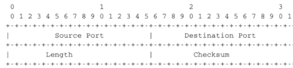
Figure 3.18: UDP Header Format
