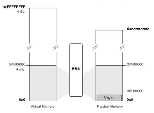
This model is simple: the first virtual memory page coincide to the first page in physical memory, the second page coincide to the second page on physical memory and so on ...
