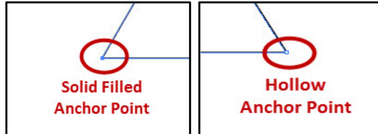
Figure 16: Solid Filled and Hollow Anchor Points
