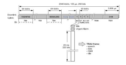
Fig. 7: GSM Abis Interface, PCM timeslot layout
