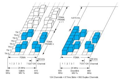
Fig. 4: GSM Air Interface, TDMA frame
