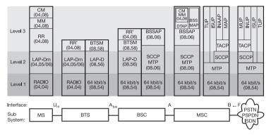
Fig. 3: OSI Layer structure in GSM
